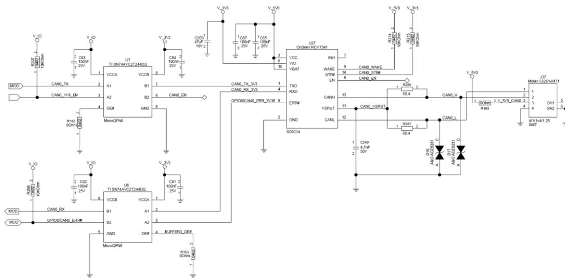
Figure 31 CAN Bus circuit example
