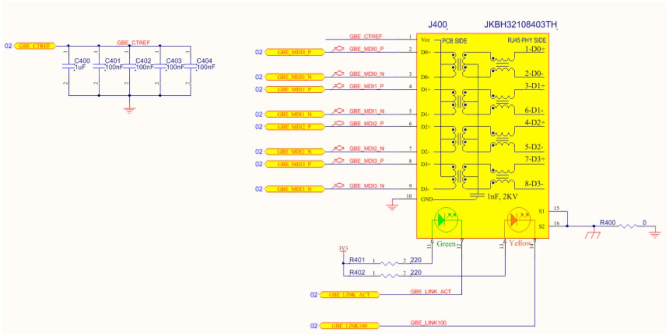
Figure 18 Ethernet 10/100/1000 Mbps standard circuit
