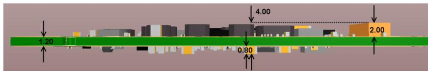
Figure 36 IGEP™ SMARC iMX6 Lateral view Widths Dimensions
