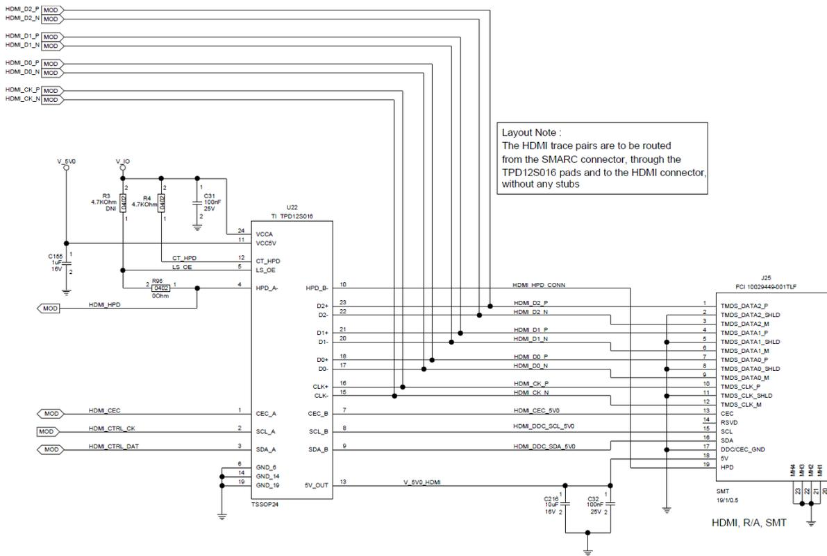
Figure 27 HDMI connection example
