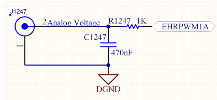
Figure 33 PWM example: RC filter
