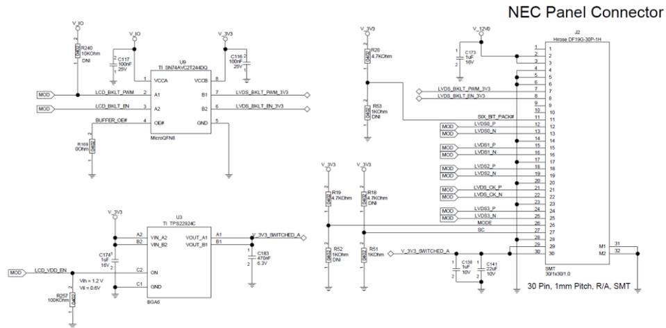
Figure 26 LVDS connection example
