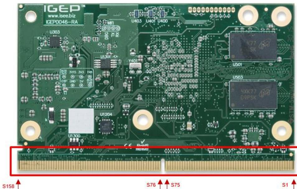
Figure 13 SMARC interface area (BOTTOM Side)
