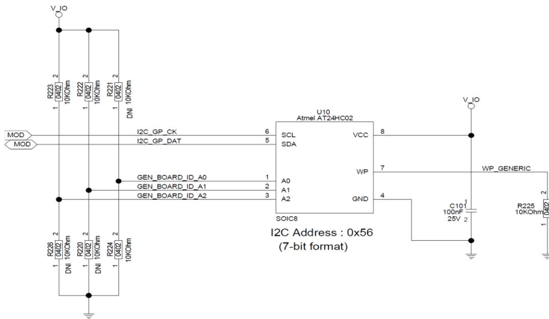
Figure 21 I2C example: EEPROM connection
