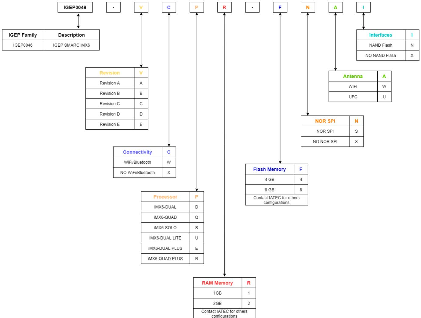
Figure 1 IGEP™ SMARC iMX6 Possible Part Number
