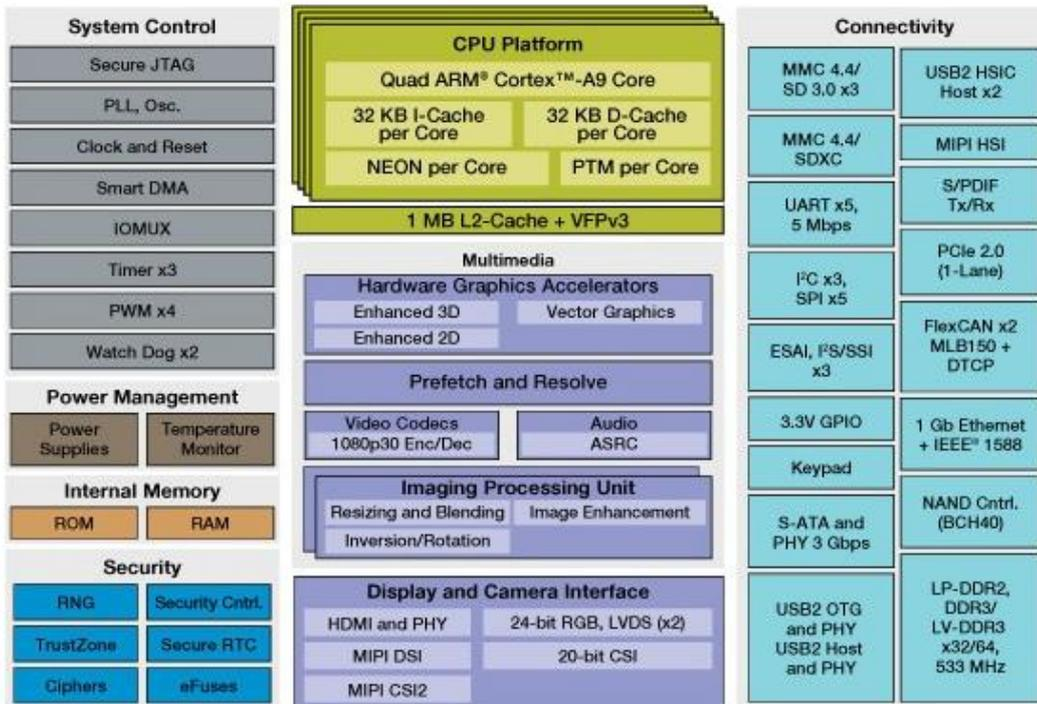
Figure 11 NXP iMX6-QUAD PLUS Processors Block Diagram
