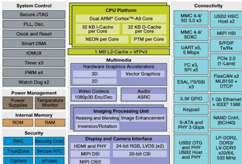
Figure 6 NXP iMX6-DUAL Processors Block Diagram
