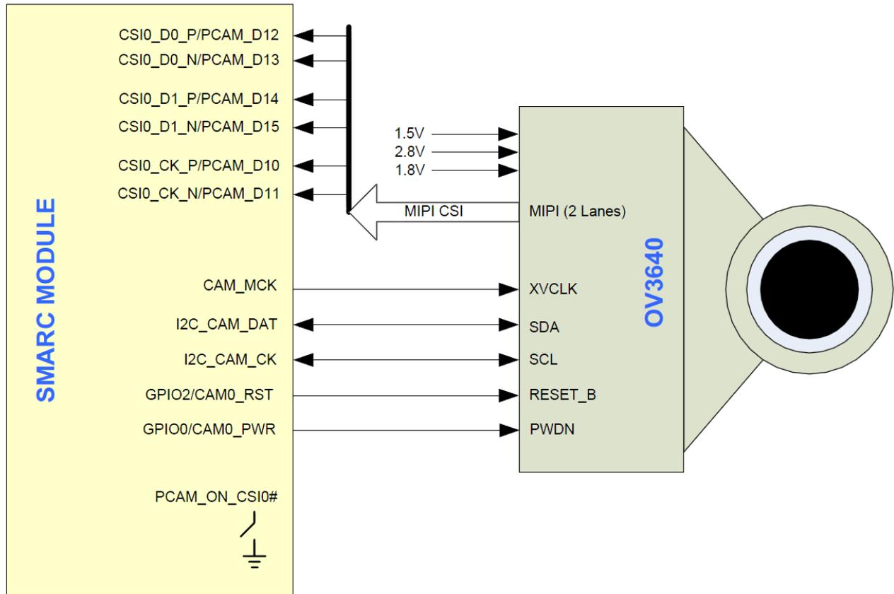
Figure 28 MIPI-CSI connection example
