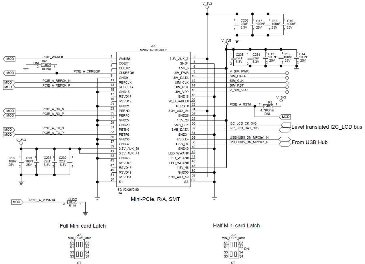
Figure 30 PCIe connection example
