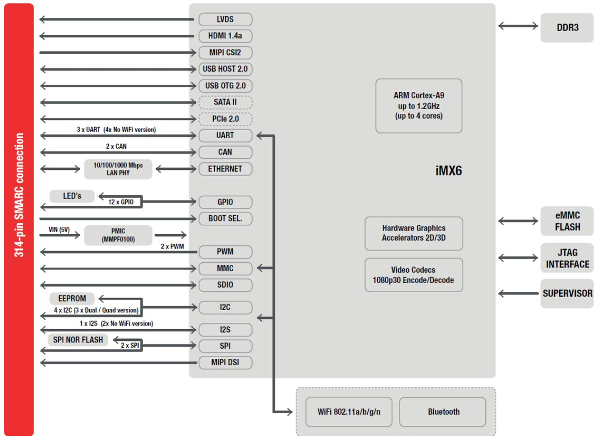
Figure 4 IGEP™ SMARC iMX6 Block Diagram
