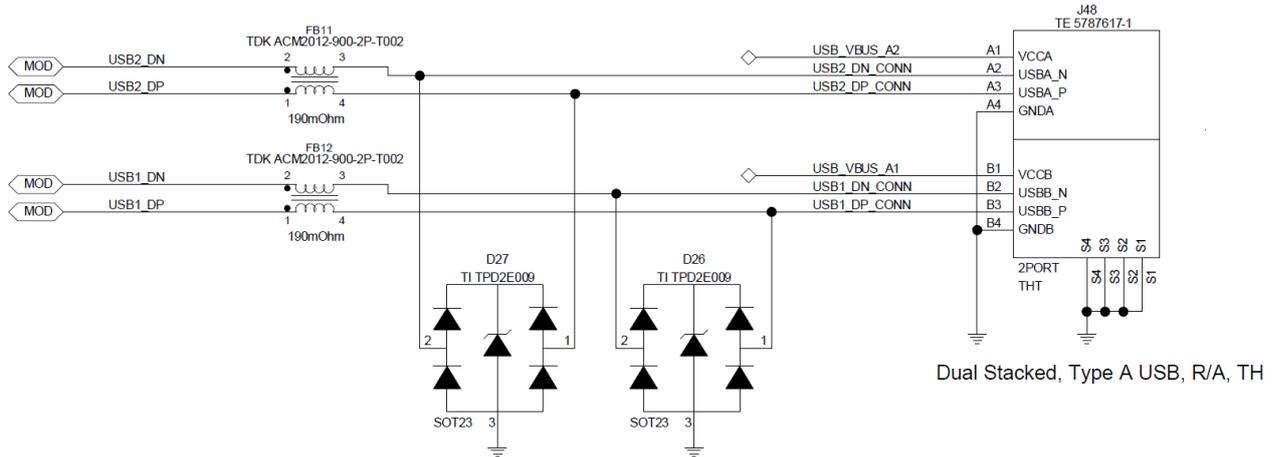
Figure 19 USB 2.0 Host connections
