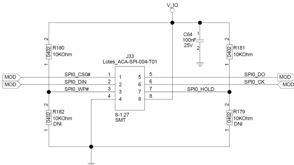
Figure 22 SPI example: SPI Flash Socket
