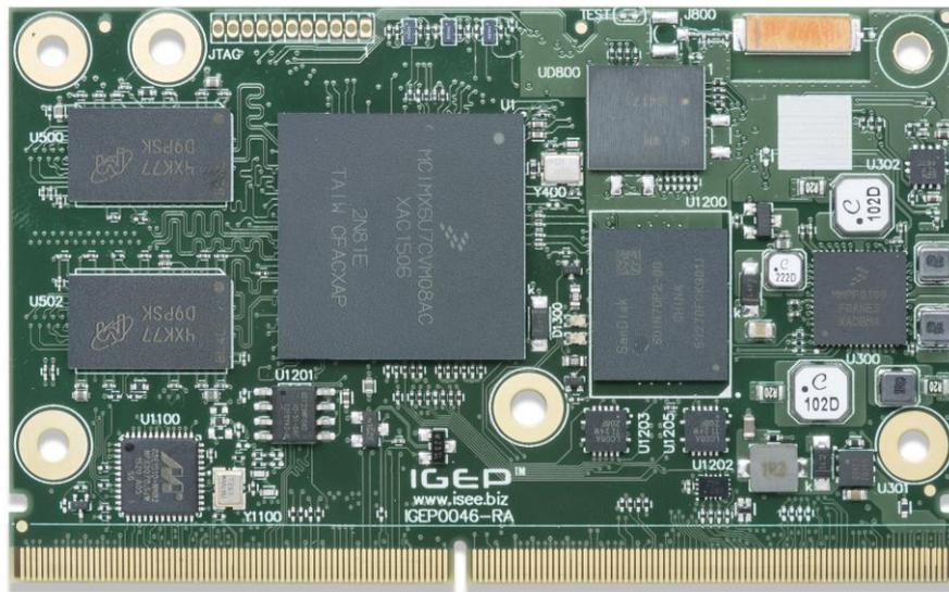
Figure 2 SMARC iMX6 – Top View
