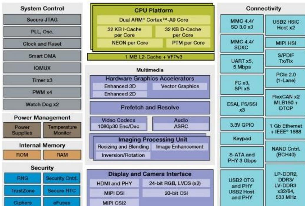
Figure 10 NXP iMX6-DUAL PLUS Processors Block Diagram
