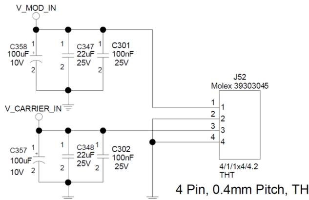
Figure 15 Power Supply Input circuit
