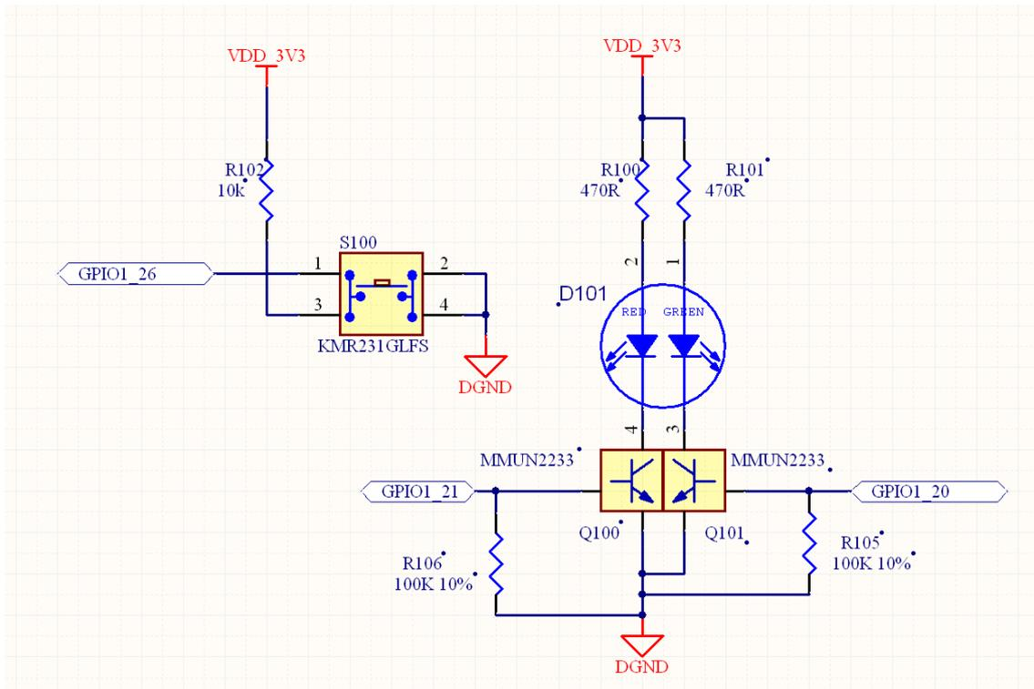
Figure 32 GPIOs example: control circuit to manage LEDs
