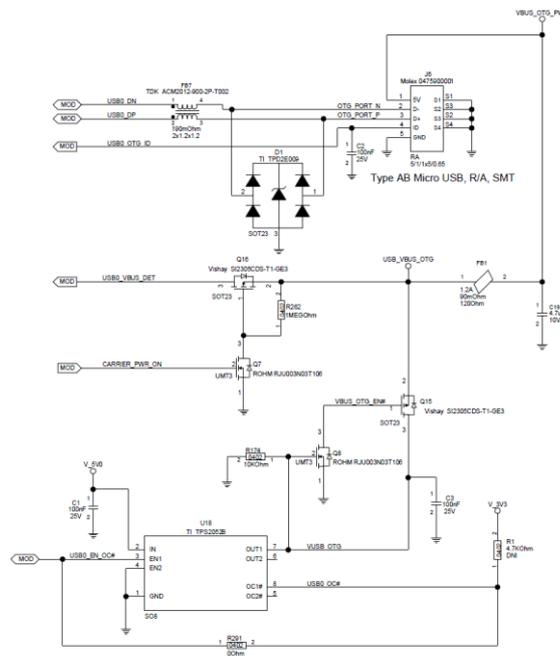
Figure 20 MicroUSB AB 2.0 OTG connections
