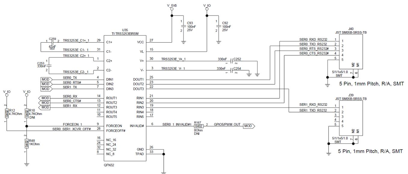
Figure 24 UART SMARC connections
