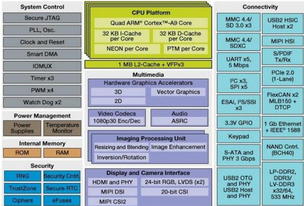
Figure 7 NXP iMX6-QUAD Processors Block Diagram
