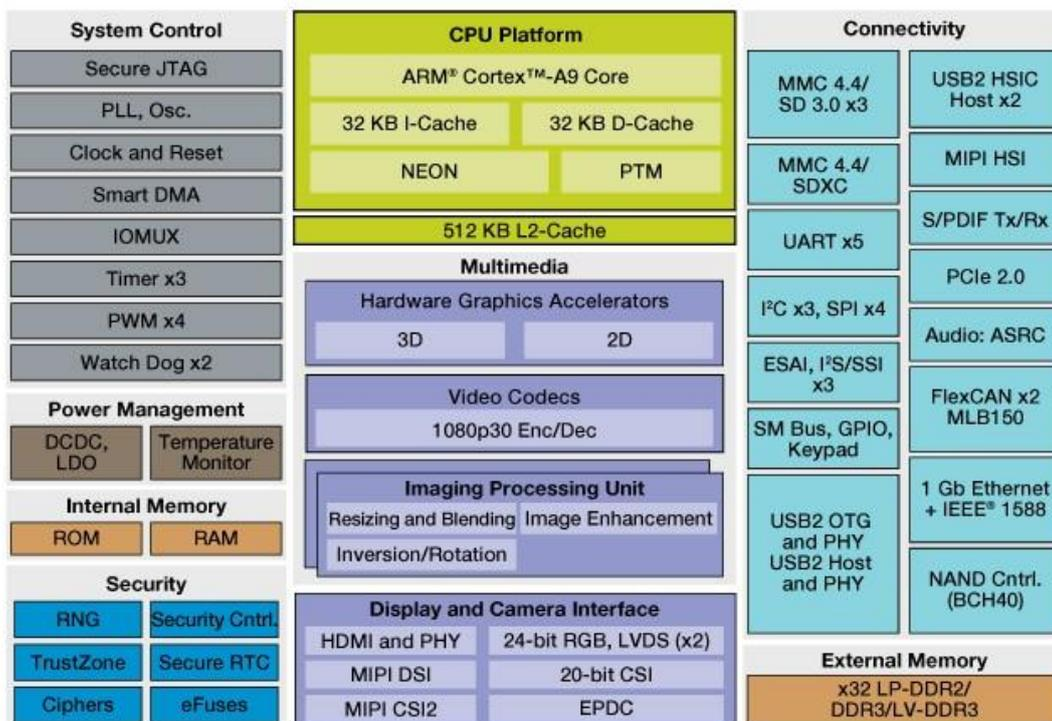
Figure 8 NXP iMX6-SOLO Processors Block Diagram
