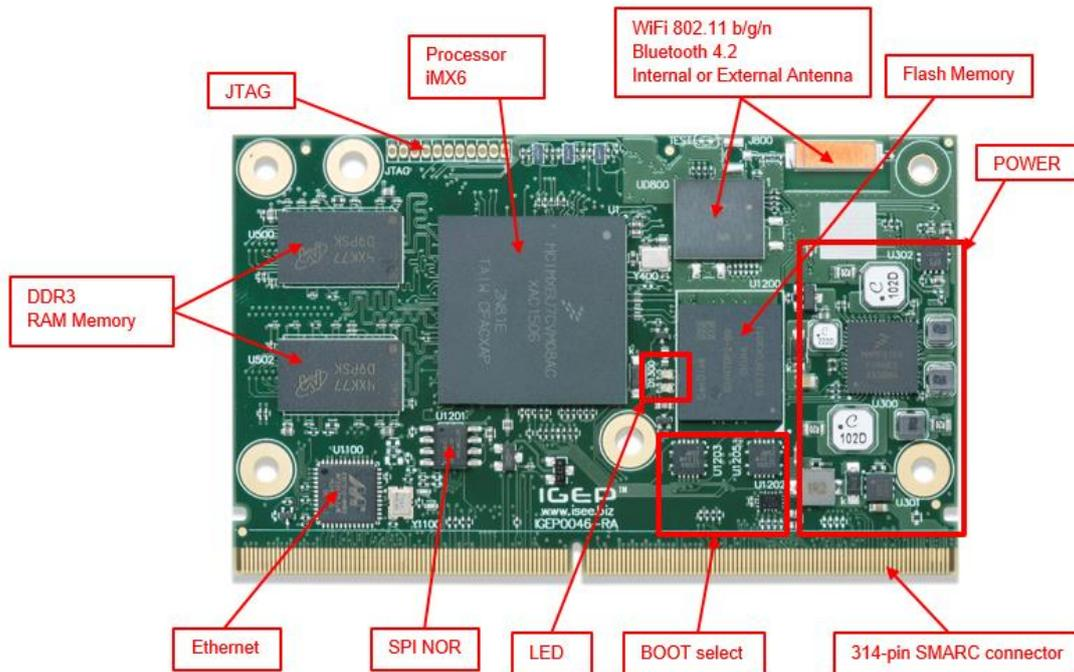
Figure 5 SMARC iMX6 Components Map
