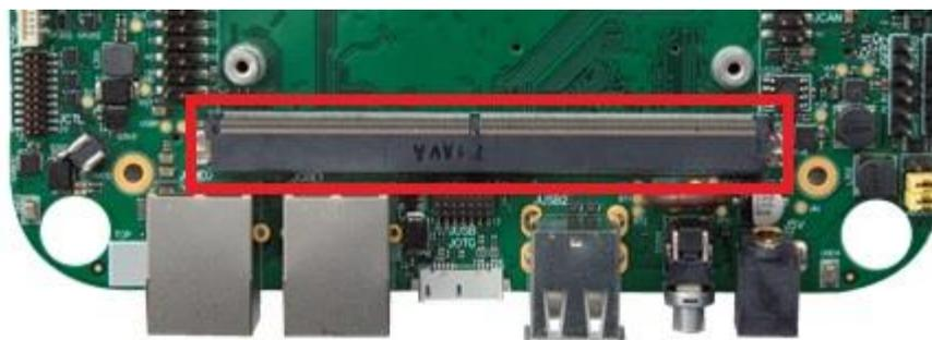
Figure 14 SMARC CONNECTOR
