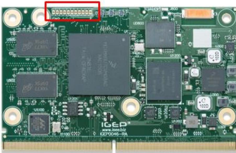
Figure 39 JTAG position in the PCB
