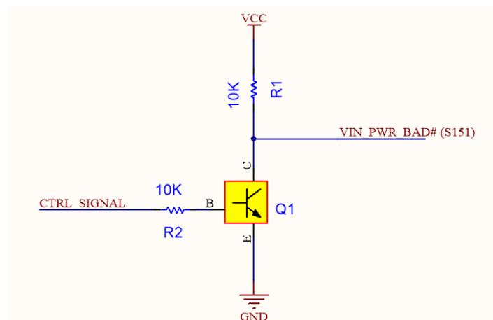
Figure 17 VIN\_PWR\_BAD circuit Example (Vcc =Vin).
