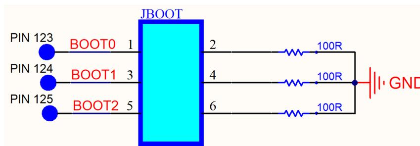
Figure 16 Boot Mode: jumpers selectors
