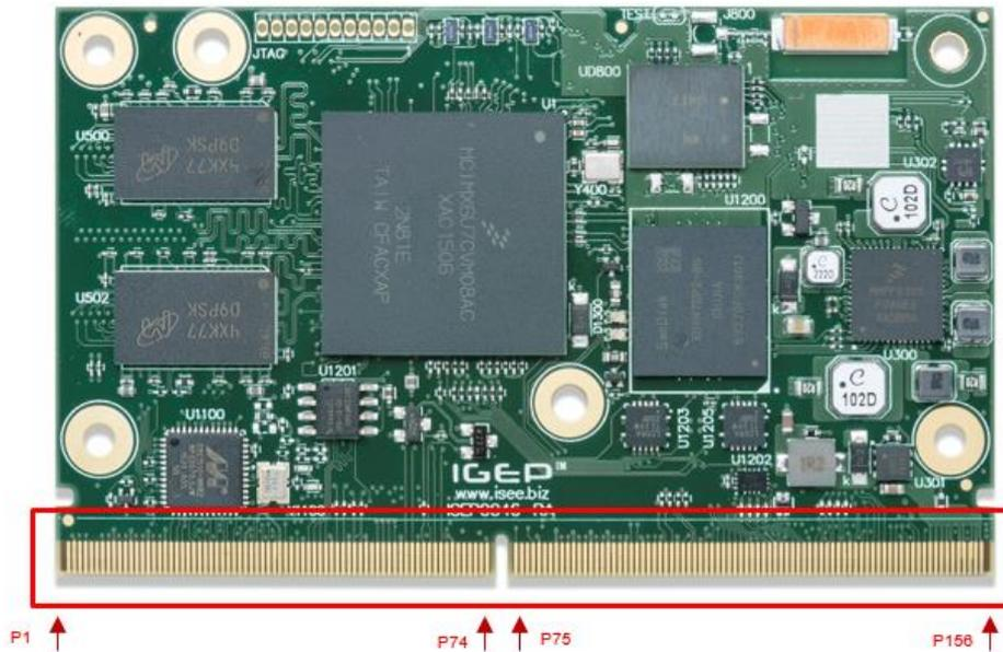
Figure 12 SMARC interface area (TOP Side)
