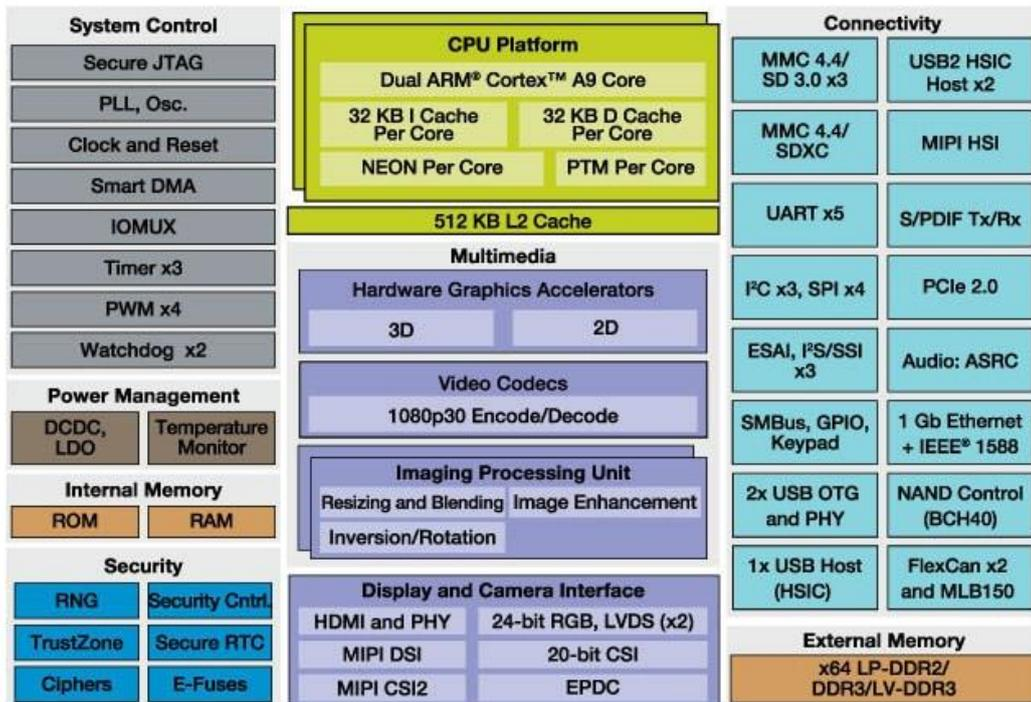
Figure 9 NXP iMX6-DUAL LITE Processors Block Diagram
