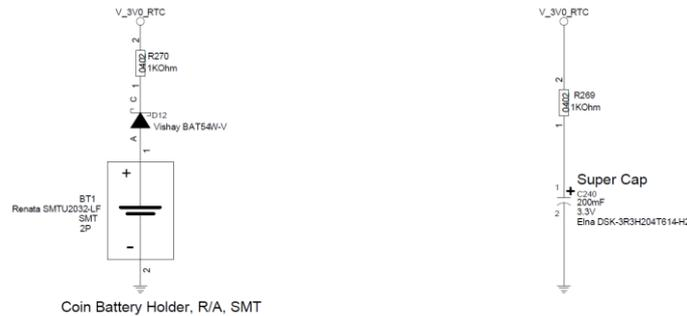
Figure 34 RTC Battery
