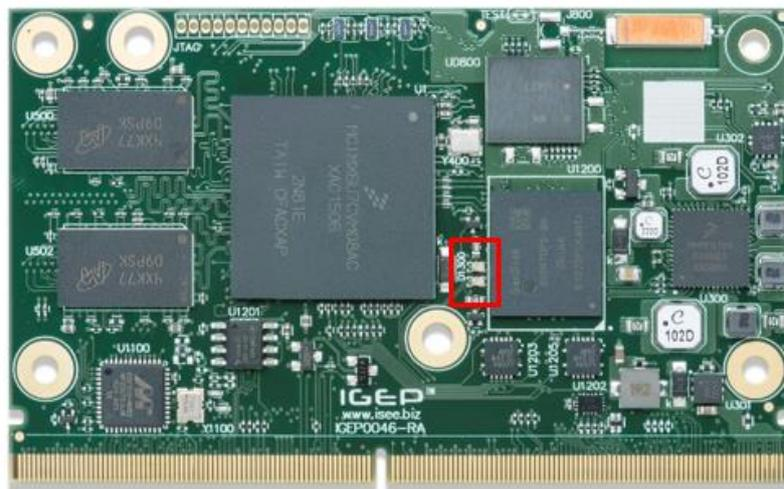
Figure 38 LEDs position in the PCB
